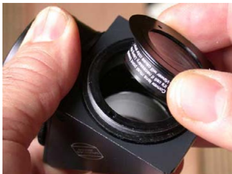
How to screw-in the glass path compensator into the Baader T2 diagonals
