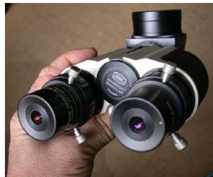
The MaxBright Binoviewer with T2 #1B Zeiss diagonal and 2" barrel (both options)
